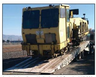
Assist in Loading with the Landoll Standard 12,000 lb. Winch (Choose a 20,000 or 30,000 lb. Winch to Load Totally Disabled Equipment)
